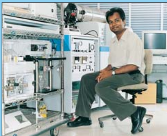
RAM SASISEKHARAN sits by a sophisticated sugar-sequencing unit. After enzymes chop up a complex sugar, advanced high-pressure liquid-chromatography equipment ( on cart ) sorts the resulting fragments, and a mass spectrometer ( right ) characterizes the building blocks in the separated pieces. Computers analyze the results from both procedures to arrive at the full sequence of simple sugars in the complex molecule.
